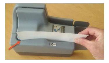
If the cleaning card is very dirty, repeat the roller cleaning process with a clean card.
